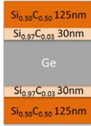
Fig. 2. Ge lifetime sample with a-Si 0.97 C 0.03 :H passivation layer and a-Si 0.50 C 0.50 :H mirror layer on both sides.
